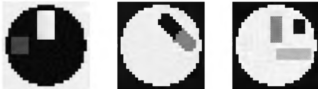
Fig. 19. Example: recovered denoised source signals. Now the SNR is even higher than in figure 18 (32, 31 and 29 dB after permutation and normalization).
