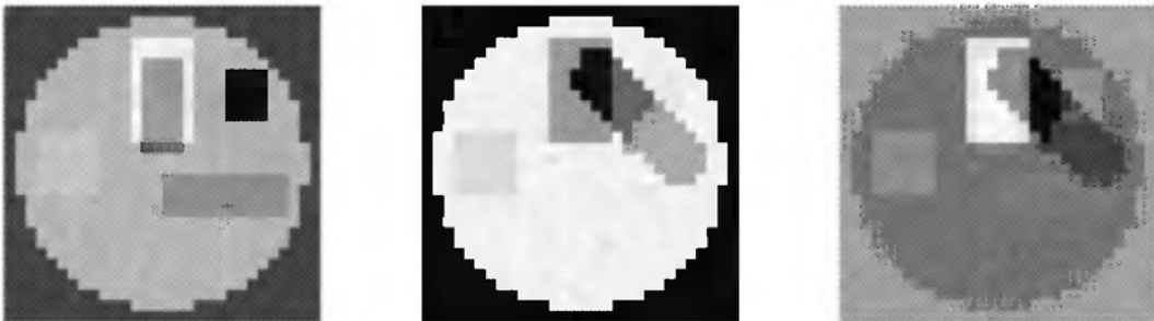
Fig. 20. Example: poorly recovered source signals using ICA. The signal-to-noise ratio between the original sources (figure 16) and the recoveries is very low with 3.3, 13 and 12 dB after permutation and normalization.
